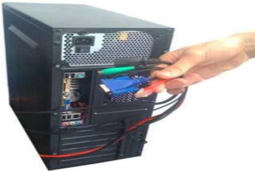
Figure 2. Disconnecting all external cables.
