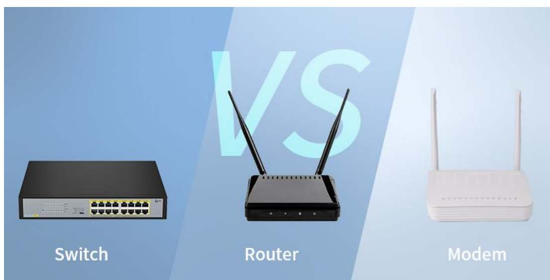
5-rasm. Switch, router, modem
